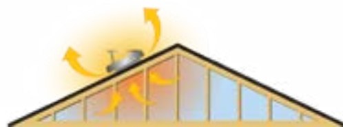
Removes Heat and Moisture from Attic Spaces
