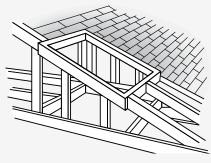
In structures that have a space between the ceiling and the roof such as an attic or crawl space, a light tunnel must be built. Nailers of 2" x 4" must be used to frame the opening between the roof header and the ceiling header. These will be used for attaching the finishing material, i.e., drywall, wall board, plywood, etc. The light tunnel should be wrapped with insulation for optimum performance. Select desired shaft and frame accordingly.
